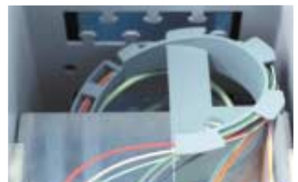
Security concept for fiber and cable protection: min. bending radius (40 mm) of pigtailed guarantees optimum transmission. Loose tube protection at insertion in and removal from mounting channel. Mechanical protection is provided by lamella.
