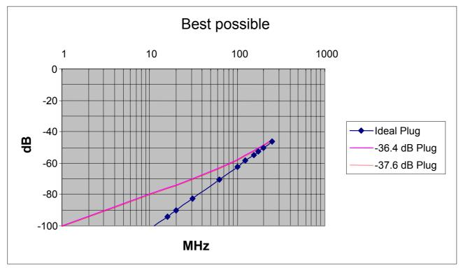
The slope for the plugs at the low and high end of the specified NEXT range for Cat. 6 change from a 20 dB / decade at lower frequencies to 40 dB / decade at frequencies above 200 MHz.
