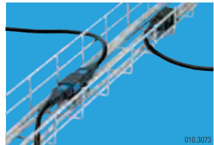
Mains cabling today: A bus-like installation from the group fuse makes the whole room accessible, this requires less cable, reduces the fire load and increases operating safety.
