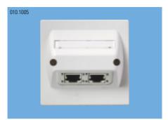
BS Faceplates are suitable for flush and surface mounting. Surface mounting requires an additional standard surface mounting box. The connection modules take up a minimum installation depth of only 10.5 mm.
