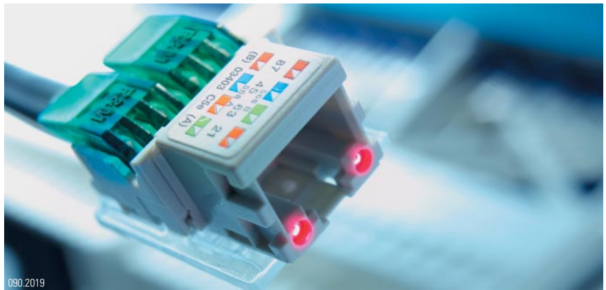
Connection module with POF (Plastic Optical Fiber)
