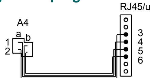
Patch Cable UTP, A4 (1) - RJ45/u (1) SRV - plug 97
